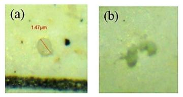
Figure 2. (a) Before and (b) after result of the hot needle test on MPs identification under the stereomicroscope.
