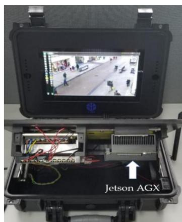
Fig. 5. Portable PD monitoring station with Jetson AGX Xavier
