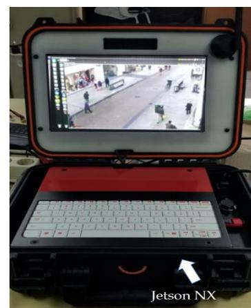
Fig. 6. Portable PD monitoring station with Jetson Xavier NX
