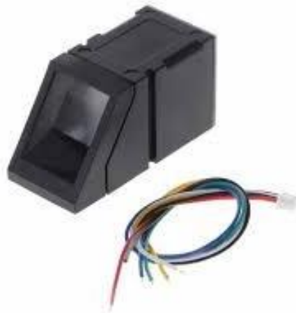
Figure 6. R307 optical fingerprint scanner [6]
