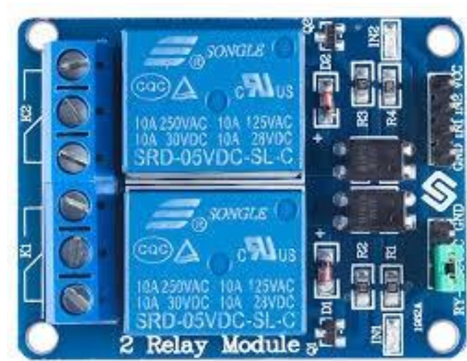
Figure 3. Two channel relay module [5]
