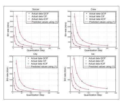
Figure 1: Actual bit-rates and predicted values using (1).
