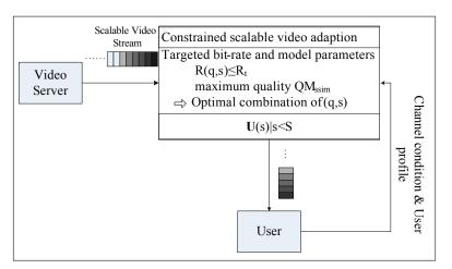
Figure 3: Constrained scalable video adaptation.
