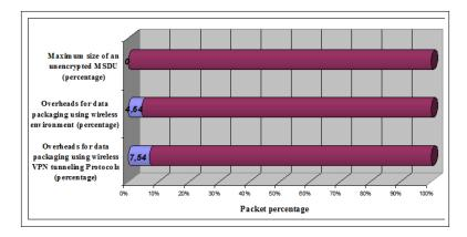
Figure 12: Overheads contribution in Wireless and Wireless VPN environment
