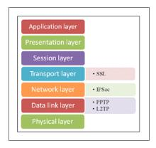
Figure 2: VPN protocols on OSI Model
