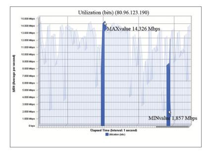
Figure 11: Min and Max values for WLAN-WLAN VPN connection
