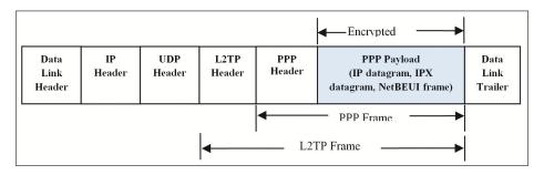
Figure 4: L2TP Tunnel Data Frame Format
