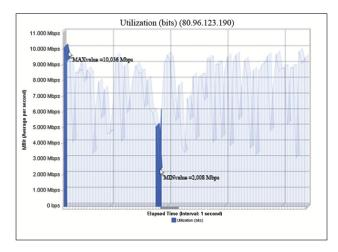
Figure 7: Minimum and Maximum values for LAN-WLAN VPN connection
