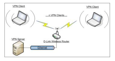
Figure 10: WLAN-WLAN VPN Connections
