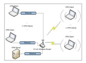
Figure 6: LAN-WLAN VPN Connections
