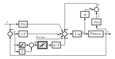
Figure 2: Control system structure with first data-driven model-free sliding mode controller [62]
