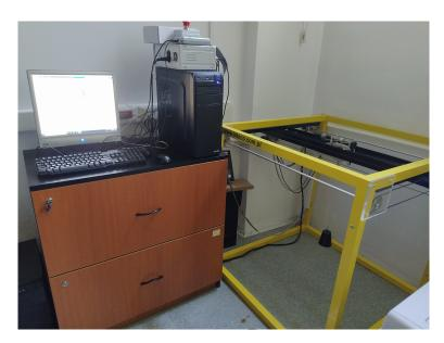
Figure 5: The experimental stand of 3D crane system laboratory equipment
