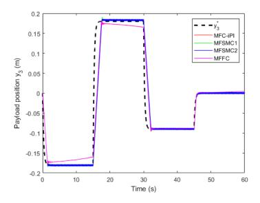
Figure 6: The experimental results of the CS with MFC-iPI, MFSMC1, MFSMC2 and MFFC controllers expressed as reference trajectory and controlled outputs (payload position) versus time
