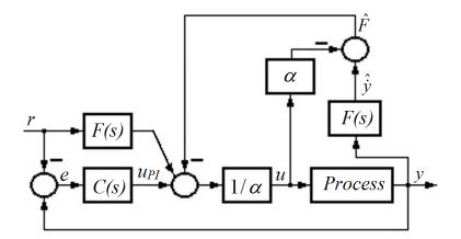
Figure 1: MFC structure with iPI controller [62]
