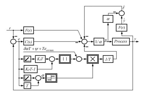
Figure 3: Control system structure with second data-driven model-free sliding mode controller [57]
