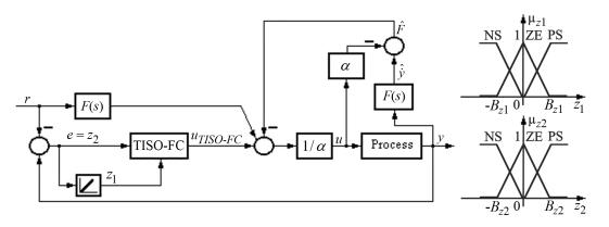
Figure 4: Control system structure with data-driven model-free fuzzy controller and input (scheduling) membership functions
