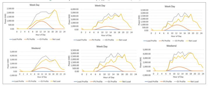
**Figure 6:** (a-c) Load profile for three schemes with BESS installation for 30% peak reduction: Net load (blue) was EV load excluding PV profile, whereas net load with ESS (orange) was derived from net load - ESS
