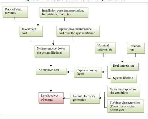
Figure 3: Methodology to estimate the wind energy production cost
