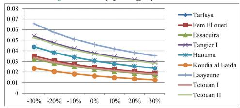
Figure 9: Effect of varying the project lifetime on the LCOE
