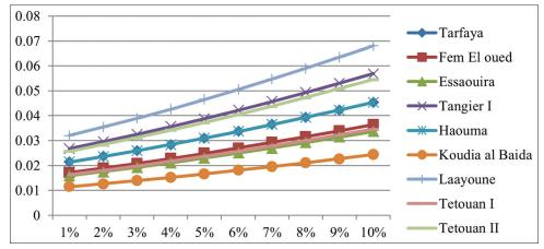
Figure 7: Effect of varying O&M on the LCOE
