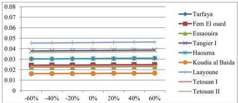
Figure 8: Effect of varying the energy output on the LCOE
