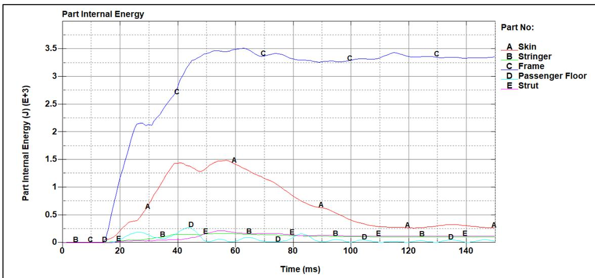
Figure 11: Internal energy plot for Aluminium fuselage at 7 m/s
