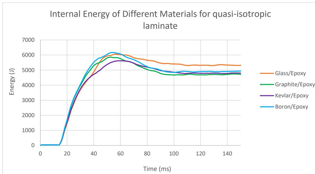
**Figure 14:** Total internal energy of fuselage made of different composite materials with quasi-isotropic laminate
