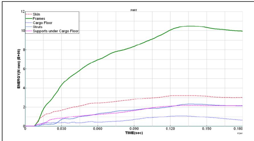
Figure 4: Energy vs time curve of each component (P. Xue et al., 2014)<sup>9</sup>
