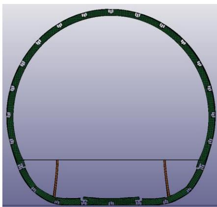
Figure 6: Aluminium fuselage after impact
