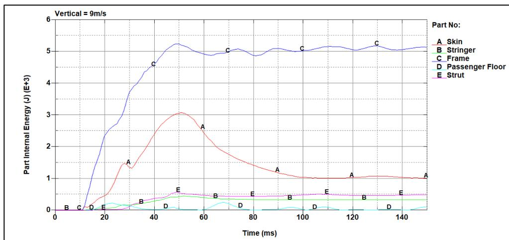
**Figure 3:** Internal energy absorbed by each component of aluminium fuselage
