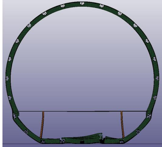
Figure 8: Graphite/Epoxy skin fuselage
