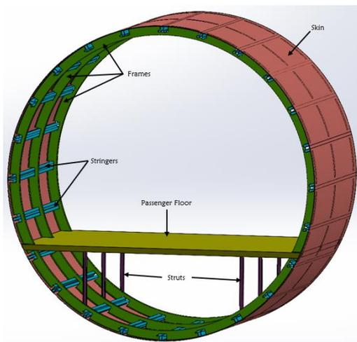
Figure 1a: Fuselage components
