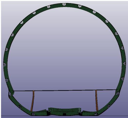
Figure 9: Kevlar/Epoxy skin fuselage
