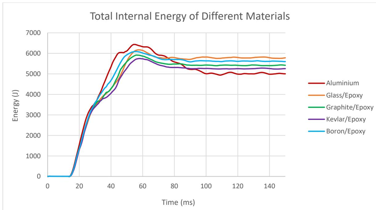
Figure 13: Total internal energy of fuselage made of different composite materials with unidirectional laminate
