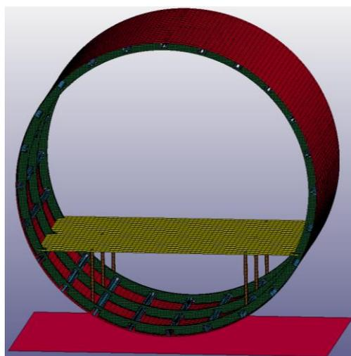
Figure 2: FE model of the fuselage and ground
