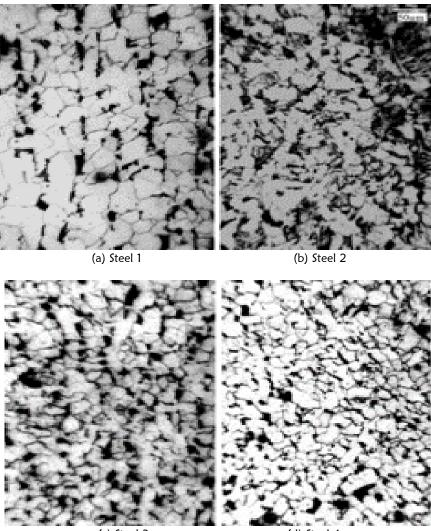
(c) Steel 3 (d) Steel 4 **Figure 6:** Optical micrograph of steels 1–4 cooled at 120°C/min (× 200).
