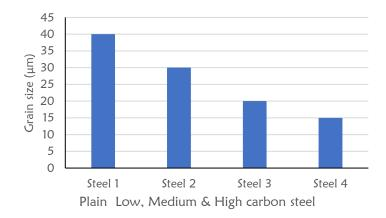
Figure 5: Average grain diameter of steels 1-4.
