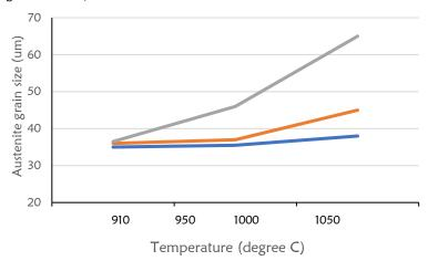
Figure 2: Variation of prior austenite grain size with temperatures for steels 1-3
