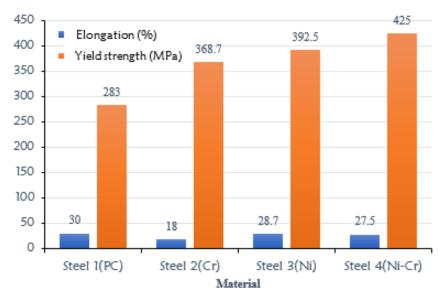
Figure 3: Comparison of yield strength and elongation of steels 1-4 cooled at 120°C/min
