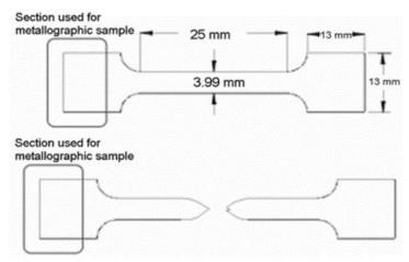
Figure 1: Dimensions of tensile specimen and location on sample for subsequent microstructure study
