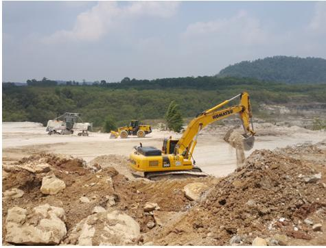
**Figure 4.** Stripping Cover Ground Layer Using 30 T Excavator
