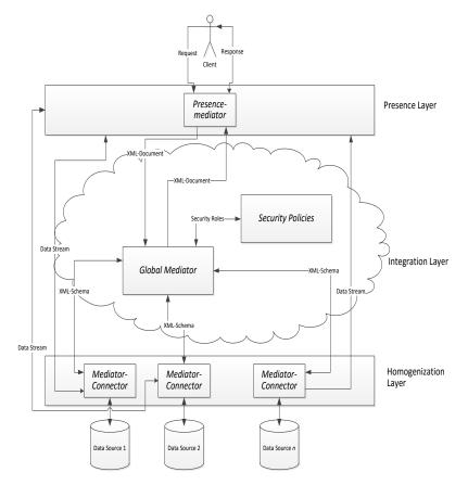
Fig. 2. 3-layer Mediation Architecture
