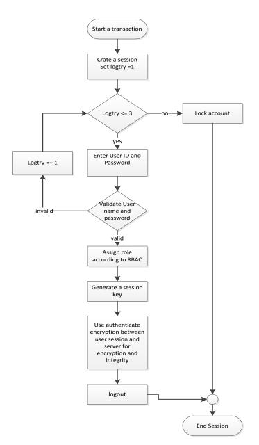
Fig. 4. Transaction Authorization Using RBAC
