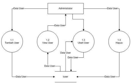
Figure 4.2 DFD Level 1 Process 1
