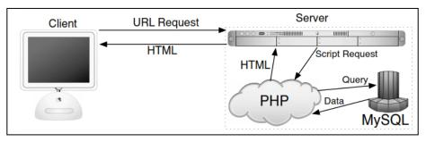
Figure 2.1 Working Process PHP and Server
