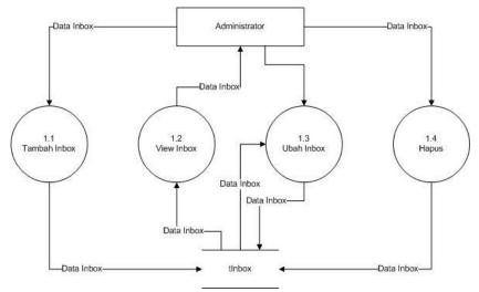
Figure 4.5 DFD Level 1 Process 4
