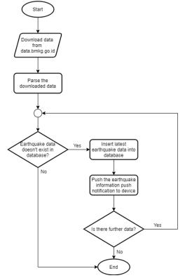
Figure 2. Earthquake Information Data Parsing Stage
