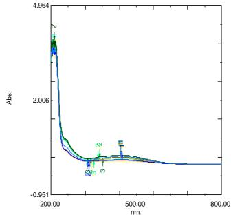
Figure. 1 The absorbance of the solution with increasing time in the synthesis of silver nanoparticles using Padina australis seaweed extract at a temperature of 70°C.
