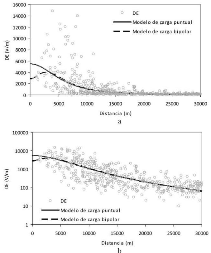
Figure 8 Electrostatic field changes  $\Delta E$  cf distance distribution for the nine thunderstorm episodes shown in Table 2. a. Lineal scale distribution b. Log scale distribution
