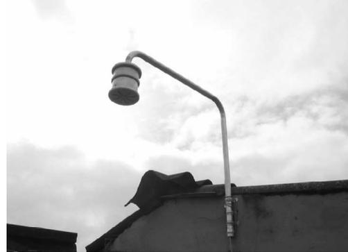
Figure 4. Electric field mill
