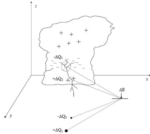
Figure 2. Bipolar charge model
