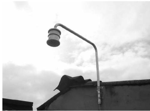
Figure. 4. Electric field mill
