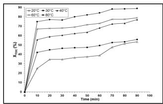
The effect of temperature on laboratory wastewater mineralization: 50 mg/L Fe(II)]0, 50 mM [H<sub>2</sub>O<sub>2</sub>]0, pH=2.8
