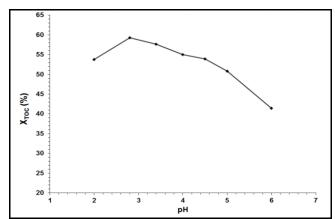
Figure 1. The effect of pH on laboratory wastewater mineralization: 50 mg/L Fe(II)]0, 50 mM [H<sub>2</sub>O<sub>2</sub>]0, T= 20°C
