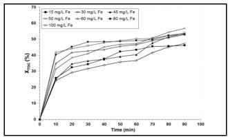
3. Iron concentration effect on laboratory mineralization: pH= 2.8, 50 mM  $[H_2O_2]0$ , T= 20°C
