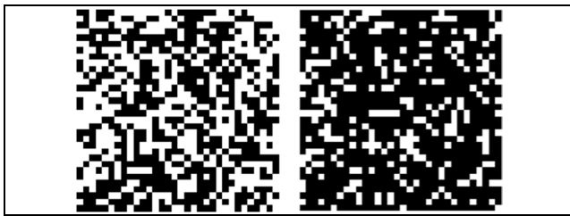
Figure 2. Two coded apertures with different transmittance levels. White pixels allow the light to pass through, while black pixels block the light
