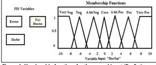
Figure 4. Membership functions for the second input (DerSat)
