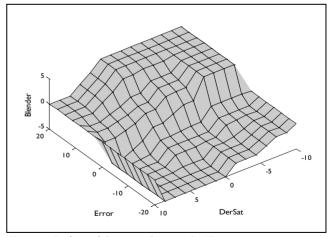
Figure 6. Surface of the control system in 3D
