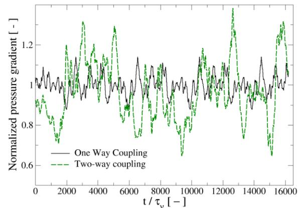
Figure 8. Time evolution of normalized pressure gradient for the one-way and two-way coupling scenarios
