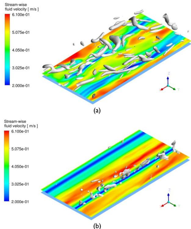
**Figure 5.** Illustration of the velocity field in the plane  $z^+ = 18$  within the buffer layer. The turbulent structures identified by the Q criterion are included. a) Single phase flow,  $Q = 50 \text{ s}^{-2}$ ; (b) two-phase flow,  $Q = 10 \text{ s}^{-2}$ . Flow is in the positive x-direction.
