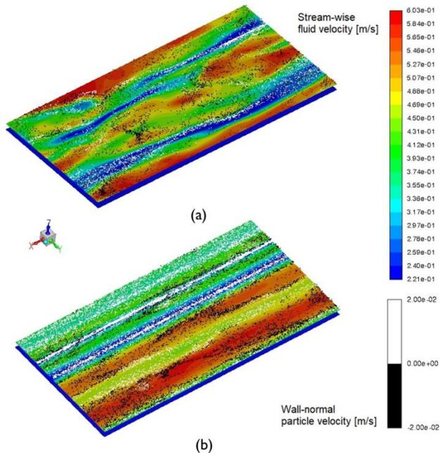
**Figure 6.** Illustration of the velocity field in the plane  $z^+ = 18$  within the buffer layer under one-way coupling (a) and two-way coupling (b) configurations. Positions of particles around that plane are shown as colored dots. Black dots represent particles moving towards the wall, whereas white dots denote particles escaping from the wall. Flow is in the positive x-direction.
