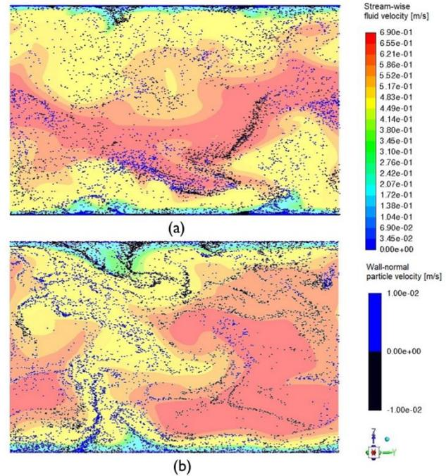
**Figure 7.** Illustration of the stream-wise velocity field in the middle stream-wise plane under one-way coupling (a) and two-way coupling (b) configurations. Positions of particles around that plane are shown as colored dots. Black dots represent particles with negative wall-normal velocities, whereas blue dots denote particles with positive wall normal velocities. Flow is orthogonal to the plane.
