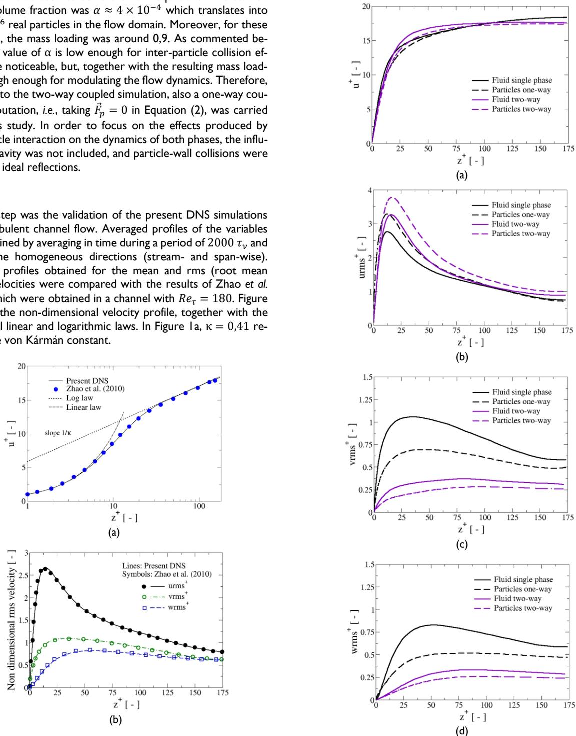
**Figure 2.** Non-dimensional fluid and particle mean and fluctuating velocities for one-way and two-way coupling conditions: a) stream-wise mean velocity, b) stream-wise rms velocity, (c) span-wise rms velocity, (d) wall-normal rms velocity
