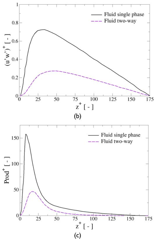
**Figure 4.** Non-dimensional fluid turbulent kinetic energy (a), turbulent shear stresses (b), and turbulent kinetic energy production term (c) for single phase and two-way coupling conditions
