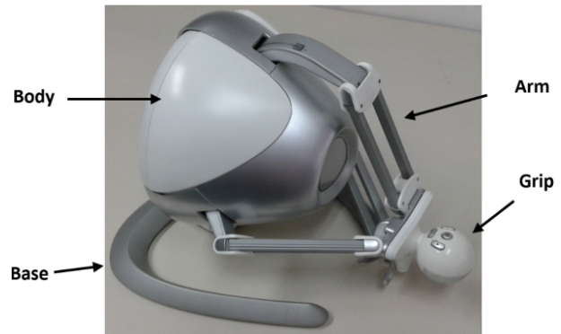
Figure 3. Kinesthetic interface Novint Falcon Source: Authors
