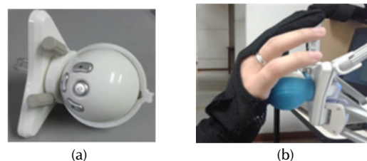
Figure 4. a) Grip adaptation of the kinesthetic interface, b) coupling between HaptTech and the Novint Falcon interface Source: Authors
