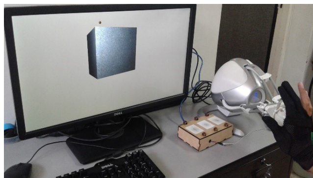
Figure 5. Scenario for experiment 3, including kinesthetic and vibrotactile stimuli
