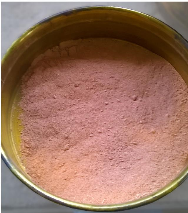
**Figure 2.** Crushed brick dust
