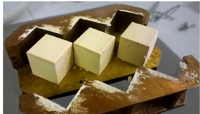
**Figure 6.** Elaboration of the mortar cubes
