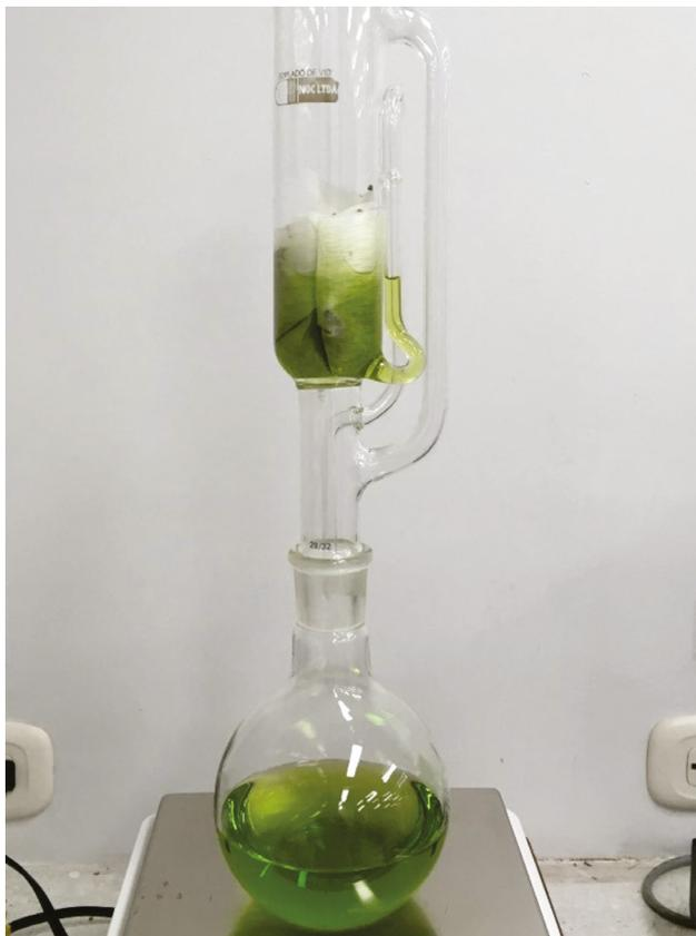
**Figure 1.** Soxhlet process to obtain compounds from cannabis biomass
