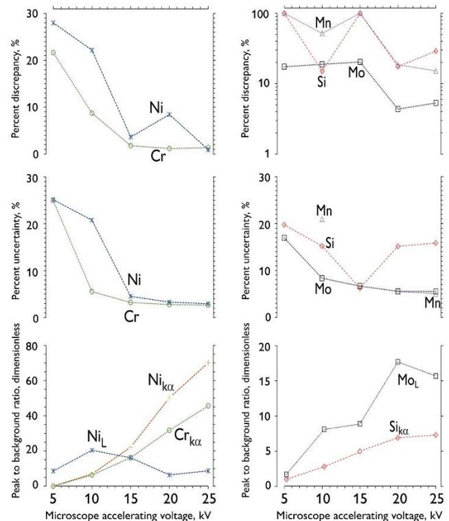
**Figure 2.** Effects of  $V_0$  variations on the discrepancy and uncertainty of the assessed elemental composition and the S-to-N ratio of spectral peaks. Left: major elements; right: minor elements. Beam intensity: 12 (a.u.); spot size: 150 nm; WD: 15 mm; and live time: 60 s.
