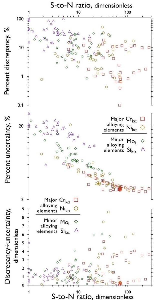
**Figure 7.** Effects of variations in the S-to-N ratio on the percent discrepancy, the percent uncertainty, and the ratio between discrepancy and uncertainty, putting together all the measurements made in this study
