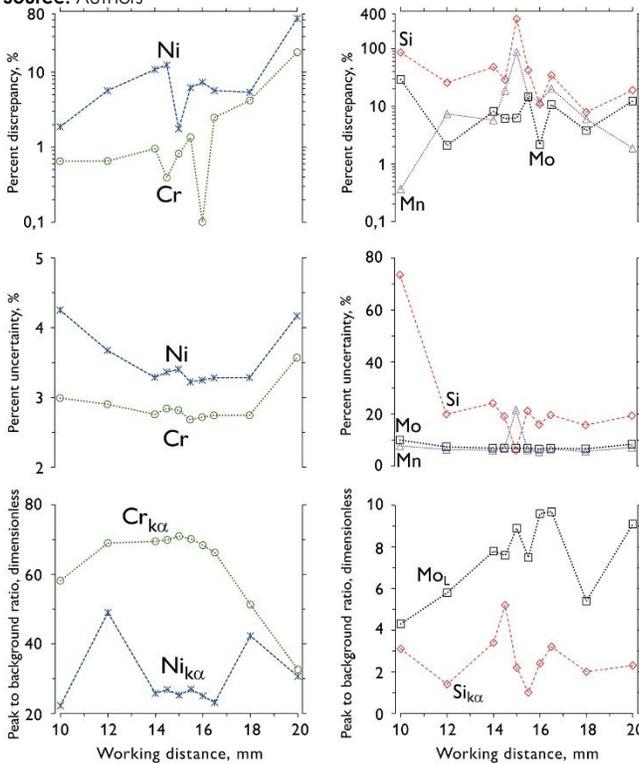
**Figure 4.** Effects of WD variations on the discrepancy and uncertainty of the assessed elemental composition and the S-to-N ratio of spectral peaks. Left: major elements; right: minor elements. Beam intensity: 12 (a.u.); spot size: 150 nm;  $V_0$ : 25 kV; and live time: 60 s.
