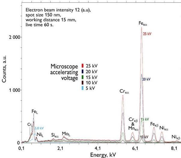
**Figure 1.** Effects of  $V_0$  variations on the energy spectra
