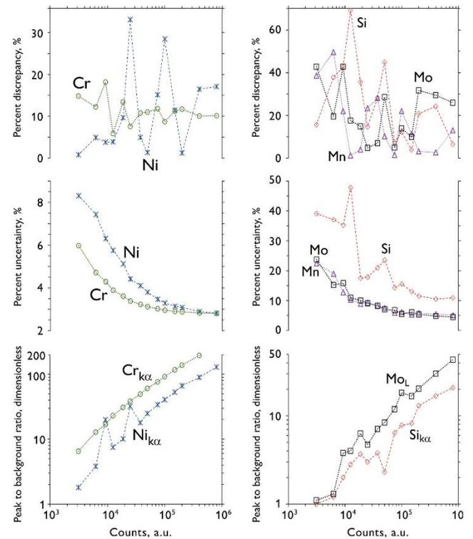
**Figure 5.** Effects of variations in the count number on the discrepancy and uncertainty of the assessed elemental composition and the S-to-N ratio of spectral peaks. Left: major elements; right: minor elements. Beam intensity: 12 (a.u.); spot size: 150 nm;  $V_0$ : 25 kV; WD: 15 mm.
