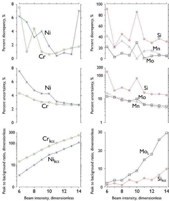
**Figure 3.** Effects of variations in the electron beam intensity on the discrepancy and uncertainty of the assessed elemental composition and the S-to-N ratio of spectral peaks. Left: major elements; right: minor elements.  $V_0$ : 25 kV; WD: 15 mm; and live time: 60 s.
