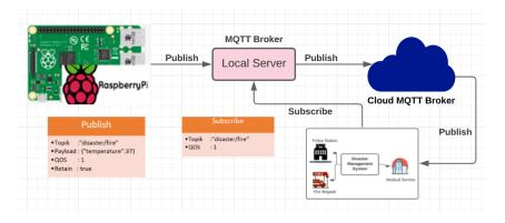
Fig. 7. MQTT Connection of the IoT, Fog and the Cloud
