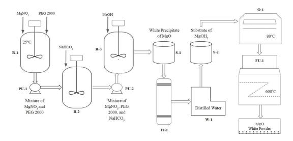
Fig. 2. Illustration of a flow chart for the manufacture of magnesium oxide nanoparticles
