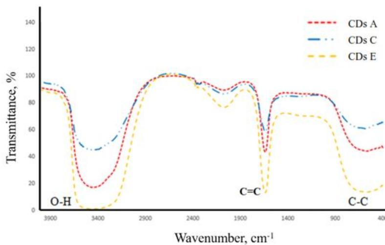
Figure 4. FT-IR spectra of CD samples.
