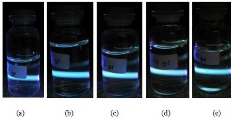
Figure 3. CDs with precursor concentrations of 0.01 g/mL (a); 0.02 g/mL (b); 0.03 g/mL (c); 0.04 g/mL (d); and 0.05 g/mL (e) exposed to UV/violet laser.
