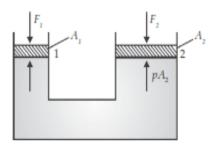
**Figure1.** The relationship between Cross-sectional Area and Hydrostatic Pressure on U Pipe Pascal's Law
