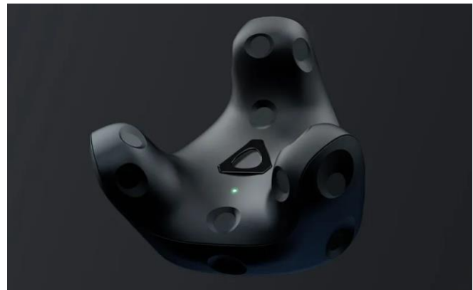
Vive Tracker , used in conjunction with the Base Station to sync the location and rotation of our physical camera with our virtual camera
