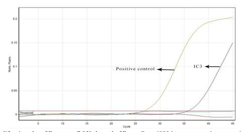
**Fig. 3.** Amplification plot of E gene on ROX channel of Rotor-Gene 6000 instrument on insect specimens using multiplex one-step qPCR along with positive and negative control
