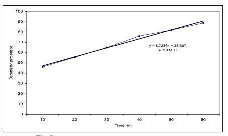
Fig. 5. Degradation percentage vs. time period for 1 mg/l
