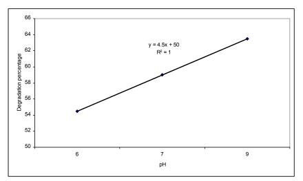
Fig. 3. Degradation percentage vs. pH for 2 mg/l
