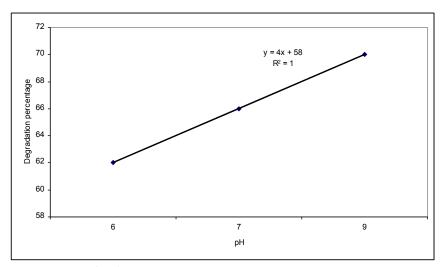
Fig. 1. Degradation percentage vs. pH for 0.5 mg/l
