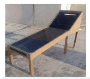
Figure 6. Fish drier diagram (Al Rawahi et al., 2013).
