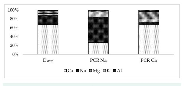
Figure 16. Main minerals in 75% ethanolic solution extract after treatment with 1:3 resin:sample ration
