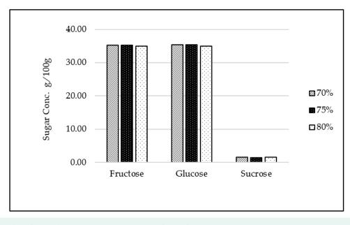
Figure 2. Effect of ethanol concentration on extraction of sugar from Fard dates.
