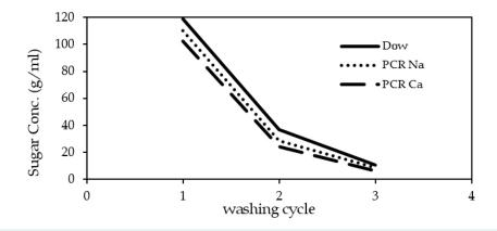
Figure 14. Sugar concentration in each washing cycle for each resin
