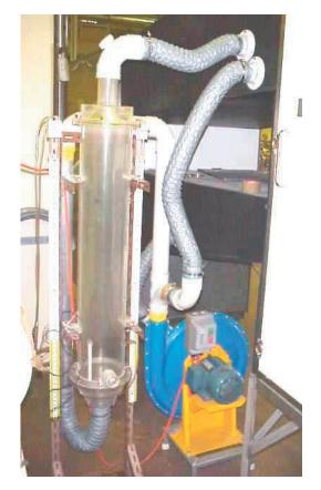
Figure 1. Fluidised bed drying experimental setup.
