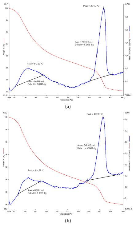
Fig. 4. ATD Thermogram of cement paste (a) - control, (b) - containing 10% MK after 3 days of hydration.
