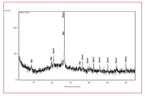
Fig. 1. Mineral phases of metakaolin by DRX.
