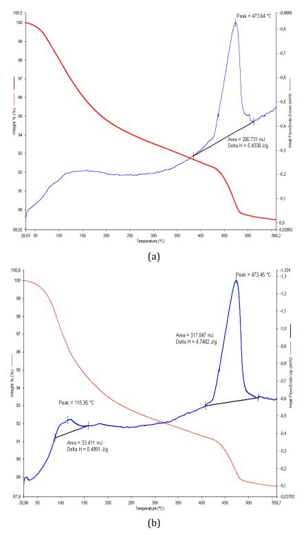
Fig. 3. ATD Thermogram of cement paste (a) - control, (b) - containing 10% MK after 24h of hydration.
