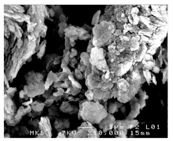
Fig. 2. Morphology of metakaolin by SEM (x10000).
