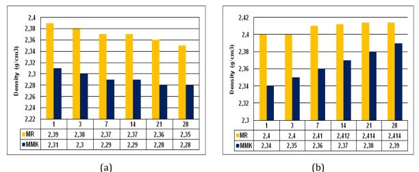
Fig. 5. Evolution of the density of (a) - Dried mortars, (b) - Wet mortars.
