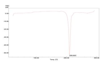
Fig. 6 DSC thermogram of pure baclofen.
