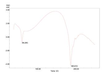
Fig. 7 DSC thermogram of F3 extrudate.
