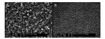
Fig. 2 SEM images of the morphology of coating that show microbead-and-nanofiber structure of EHDA (a) and micro/ nanoporous (b) structure of spin coatings.
