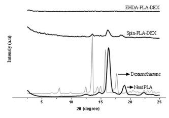
Fig. 1 X-ray diffractograms of neat PLA, dexamethasone, Spin-PLA-DEX and EHDA-PLA-DEX.
