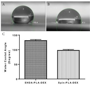
Fig. 5 The images (a and b) and numerical values (c) of water contact angles of samples.
