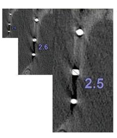
Fig. 6 Linear measurement of pin diameters at 100%, 200% and 400% magnifications.
