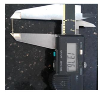
Fig. 1 **Pin length measurement by digital caliper.**
