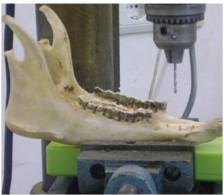
Fig. 3 Parallel drilling of implant holes.
