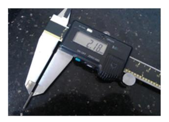
Fig. 2 Pin diameter measurement by digital caliper.
