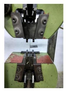
Figure 5. The peel test
