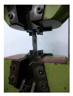
Figure 4. Shear test
