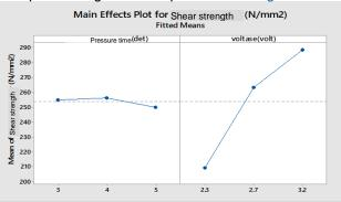
Figure 12. Main Effects Plot of shear strength
