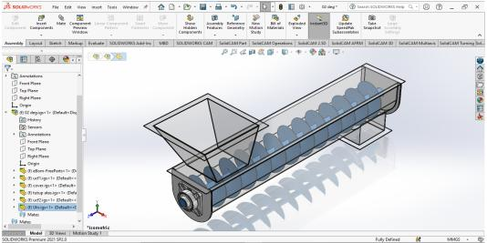
Figure 1. 3D Model of Screw Conveyor
