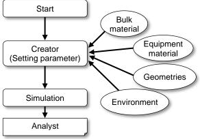
Figure 2. Flowchart of EDEM simulation
