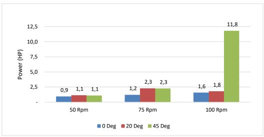
Graph 4. DEM Simulation results for horsepower
