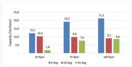
Graph 3. DEM Simulation results for capacity
