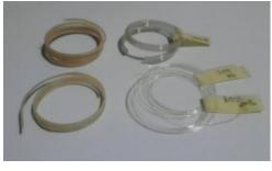
Figure 3.3 Filament produced from the mini extruder
