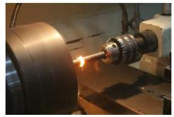
Figure 2.3 Friction Welding Process
