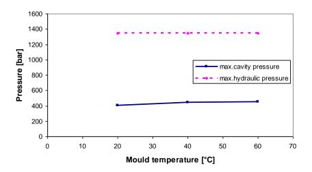
Graphic 3.3. Influence of mould temperature on max.hydraulic pressure and max.cavity pressure
