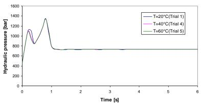
Graphic 3.2. Influence of mould temperature on hydraulic pressure profile
