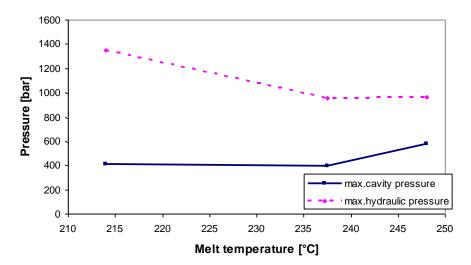
Graphic 3.8. Influence of melt temperature on maximum hydraulic pressure and cavity pressure
