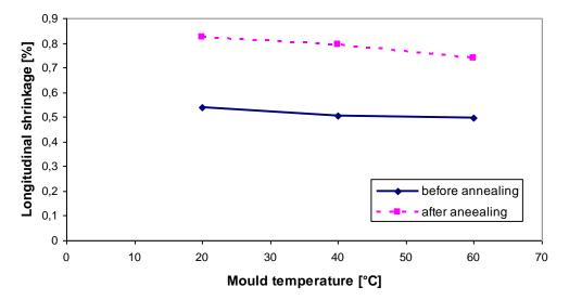
Graphic 3.5. Influence of mould temperature on longitudinal shrinkage
