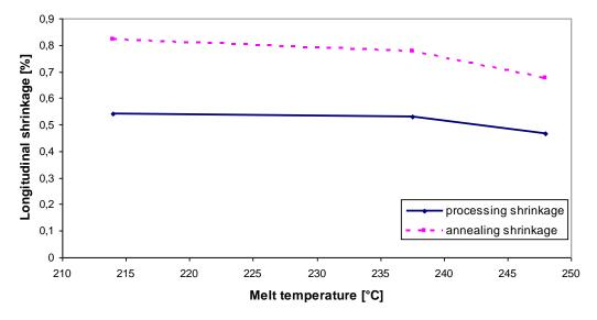
Graphic 3.10. Influence of melt temperature on longitudinal shrinkage
