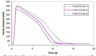
Graphic 3.1. Influence of mould temperature on cavity pressure profile
