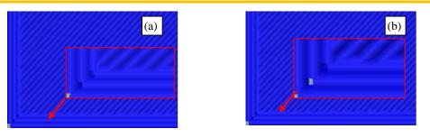
Figure 5. Gap result from slicing process with extrusion width of (a) 0.3 mm, (b) 0.4 mm
