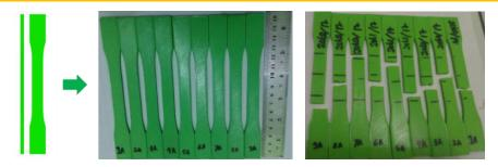
Figure 3. (a) Printed specimens (b) Tested specimens
