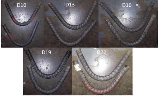
Figure 6. Pull Fin Reinforcement Steel Ben Test Results
