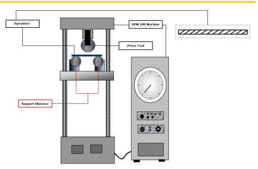
Figure 3. UPM 200 Bending Testing Machine Series
