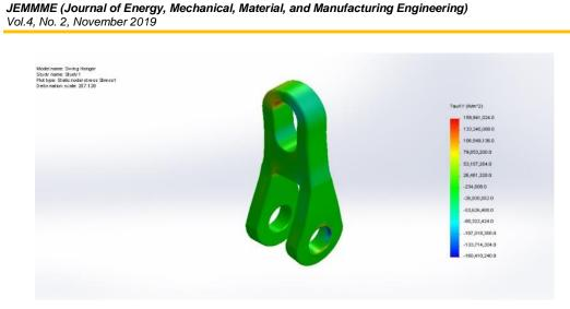
Figure 8. Shear Stress Simulation Result by Using Solidworks
