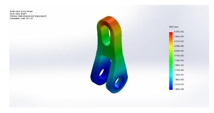
Figure 9. Strain Simulation Result by Using Solidworks
