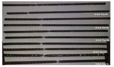
Figure 5. Pull Fin Reinforcement Steel Tensile Test Results
