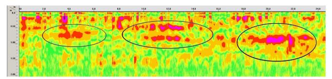
Fig. 3 Calibrated on the basis of drilling data, ground-penetrating radar cross section recorded in dry period. There is fragmented formed limestone between compact layers (marked in black) (2012)
