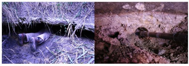
Fig. 2 Sampling at the exposure beneath the carbonate bench by using steel cylinders
