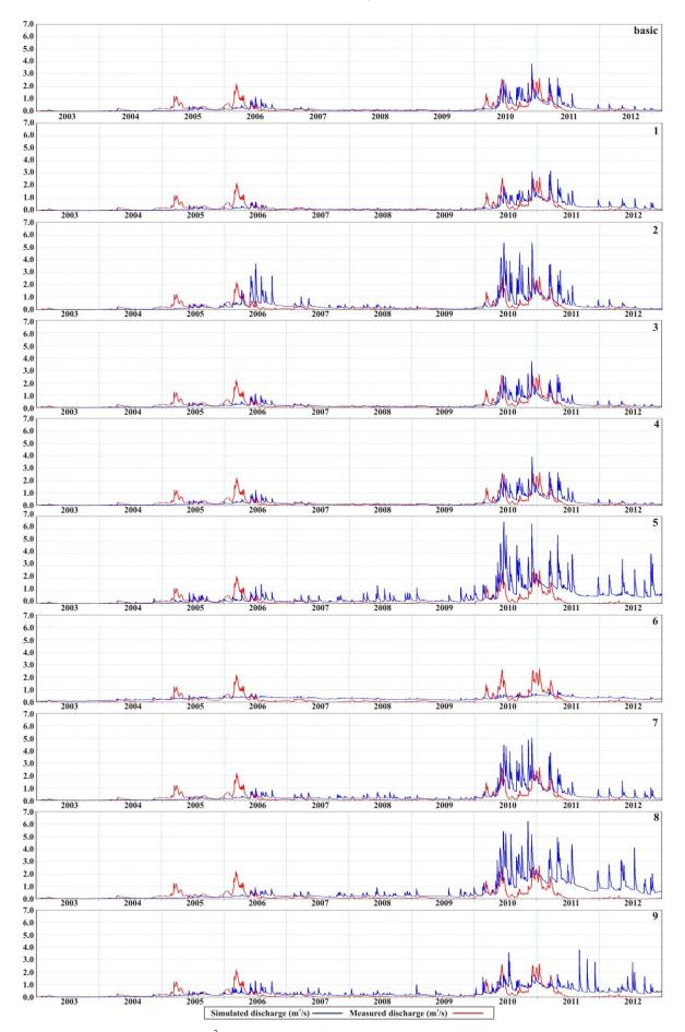
Fig.~4 Simulated discharge (m $^3$ /s) curves of the different model variations compared to the measured data series
