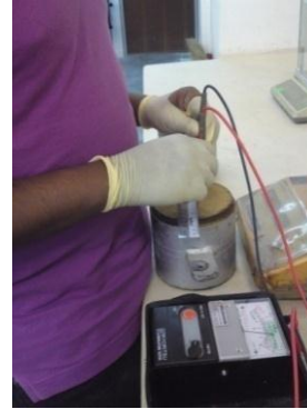
Figure 4: Measurement of electrical resistance after compaction of soil
