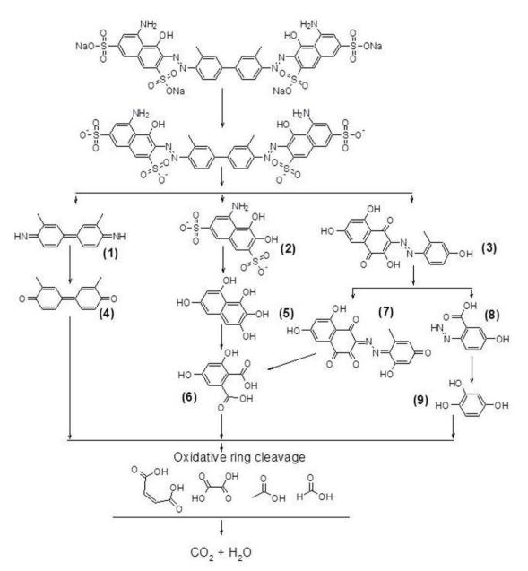
Figure 10. A possible degradation pathway of TB
