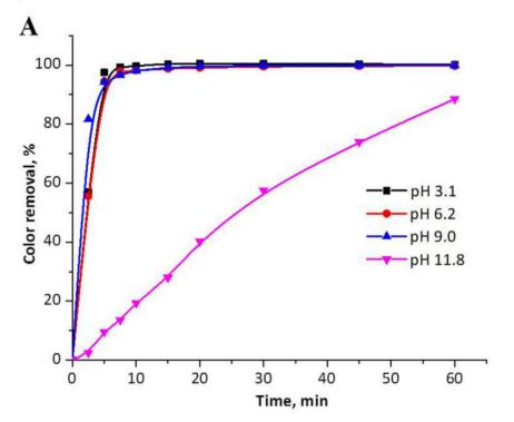
Figure 5A. Effect of pH on color removal
