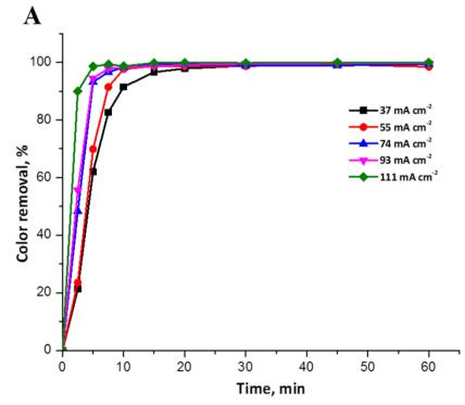
*Figure 4A. Effect of current density on color removal*
