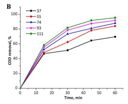
**Figure 4B.** Effect of current density on COD removal; conditions - 0.2 % NaCl, current density- 93 mA cm<sup>-2</sup>, dye – 50 mg L<sup>-1</sup>; electrolysis time – 60 min
