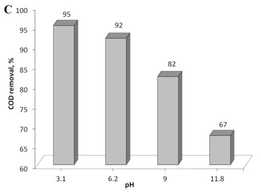
**Figure 5C.** Effect of pH on COD removal; conditions  $c_{NaCl}$ , 0.2 % (w/v), current density – 93 mA cm<sup>-2</sup>, [TB] – 50 mg L<sup>-1</sup>, electrolysis time – 60 min
