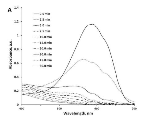
**Figure 2A.** The variation of absorption with electrolysis time. Conditions; 0.2% NaCl + 50 mg L<sup>-1</sup> TB, current density – 93 mA cm<sup>-2</sup>,  $\lambda_{max}$  = 590 nm
